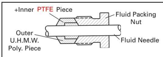
\*Apply QH-130 (Loctite #242 med. strength blue) sealing compound on threads.
